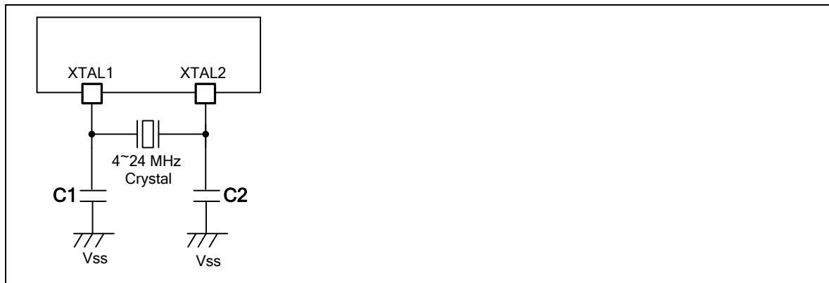
Figure 5.3-1 NM1200/NM1100 Typical Crystal Application Circuit
