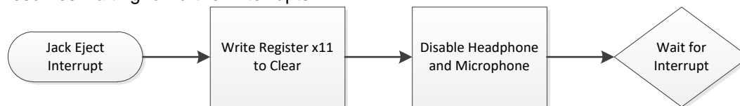
Figure 38: Jack Eject Flowchart
